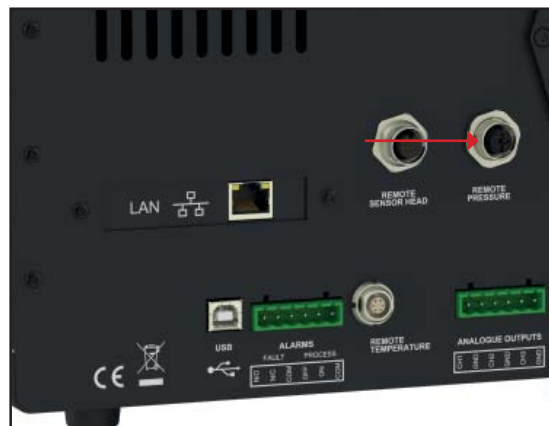
Figure 10 Remote Pressure Transducer Connection
