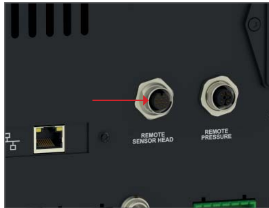
Figure 6 Dew-Point Sensor Connection
